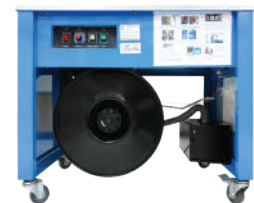
Odor and smoke absorber from semi-automated plastic strapping machine
